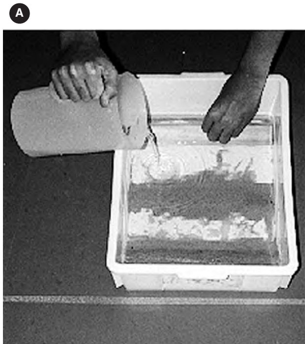
121Figure .3 How to study the effect of waves on an offshore storm bar
