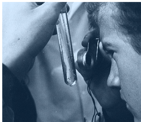
Figure 107.2 The test tube microscope
