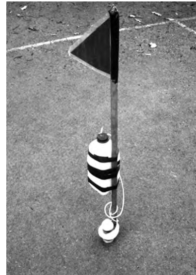
Figure 100.1 Homemade current drogue
