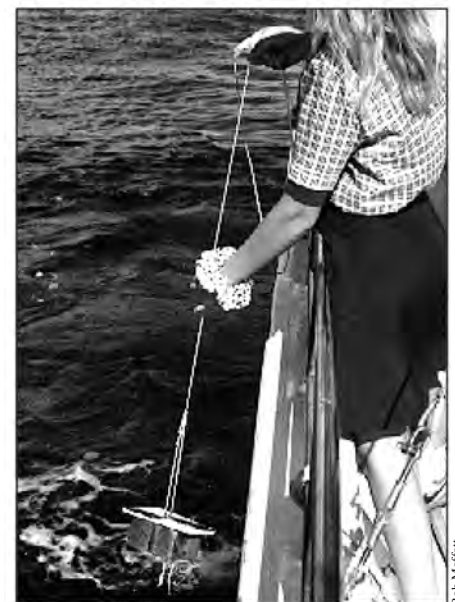
Figure 92.2 Inexpensive type of secchi disk using a brick and a ice cream container lid.
