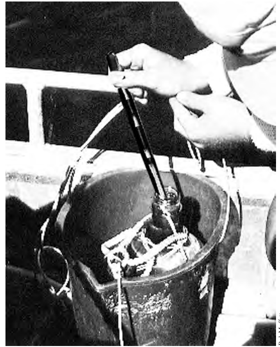
Figure 97.1 Using home made field thermometer
