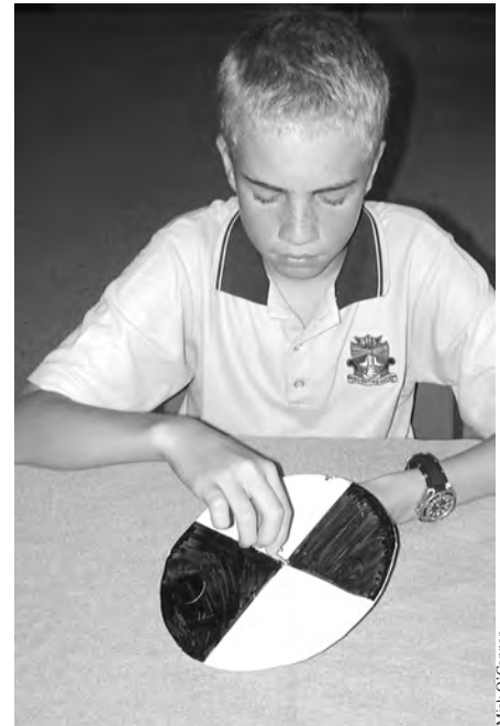
Figure 92.1 Screwing the cup hook in through the disk into the lead weights,
